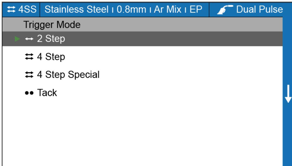
**2 Step** - Pull and hold the trigger to weld release to stop welding.
