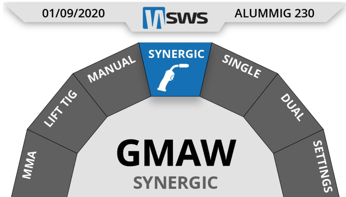
**MMA** - Stick welding mode and is used for the MMA arc welding process.
