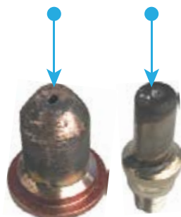
Worn Nozzle Worn Electrode
