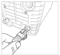
Power the receiver using the wall plug adapter.
